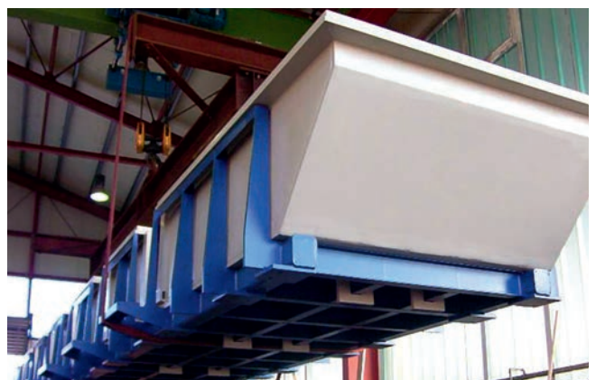
Pickling plant in PP
