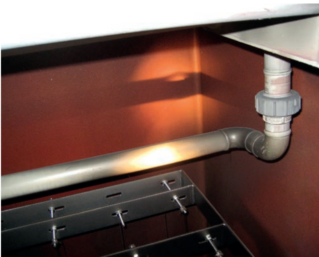
COROFLAKE coating in a wet ESP
