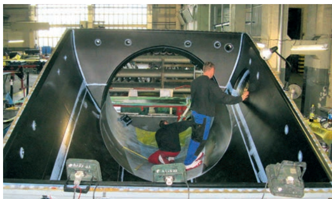
Rubber-lined water chamber
