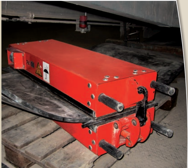
On-site operation of WK-Vulcanizing Press System
